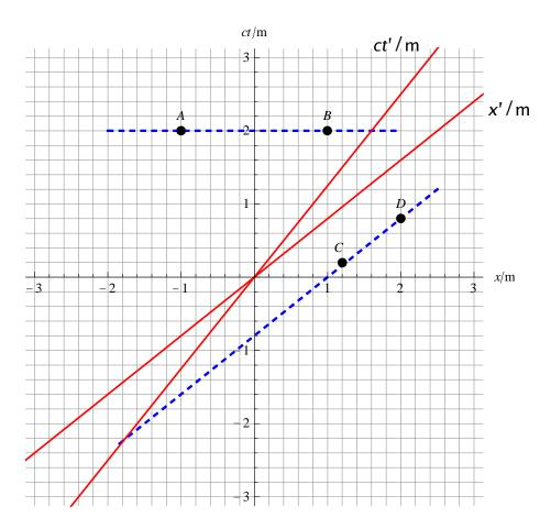
Events simultaneous in S lie on the same horizontal line (parallel to the S space axis) Hence A and B.
