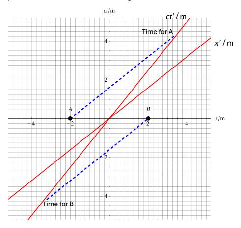
**7.** A spacecraft moves at 0.8c relative to Earth. A light signal is emitted towards the spacecraft from a space station that is 4 ly from Earth. When does the light signal arrive at the spacecraft? Answer this with a spacetime diagram and justify your answer with appropriate calculations.
