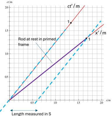
The rod has proper length 1 m. It is at rest in frame S', so it moving relative to S.
