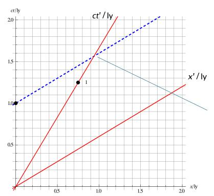
The ticks of the clock in S are apart by a time  $\Delta t$  given by  $c\Delta t=1$  ly . The clock is at rest in S so this time interval is a proper time interval. This clock moves relative to S'.
