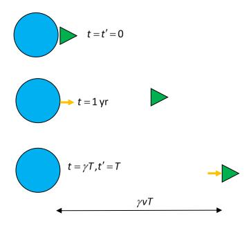
The light signal has been travelling for a time  $\gamma T-1$  to reach the spacecraft and so  $c(\gamma T-1)=\gamma Tv$ . Solving for T we get
