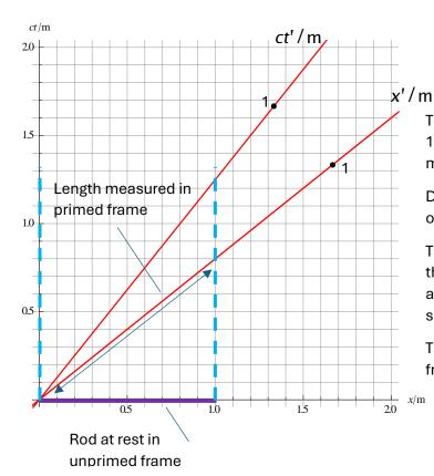
The rod has proper length 1 m. It is at rest in S so it is moving relative to S'.
