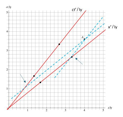
We draw lines through A parallel to the primed axes and see where they intersect the primed axes.
