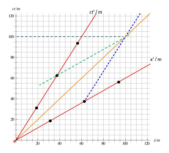
The green dotted line shows the time (× c) for the photon to get across according to the rocket. It is 50 m i.e.  $\frac{L}{c}$  as claimed earlier.
