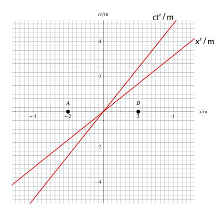
We draw lines though A and B parallel to the primed space axis. The line through B intersects the primed time axis earlier than that through A so event B occurs first.
