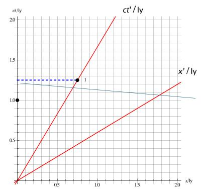
The ticks of the clock in S' are apart by a time  $\Delta t'$  given by  $c\Delta t'=1$  ly. The clock is at rest in S' so this time interval is a proper time interval. This clock moves relative to S.
